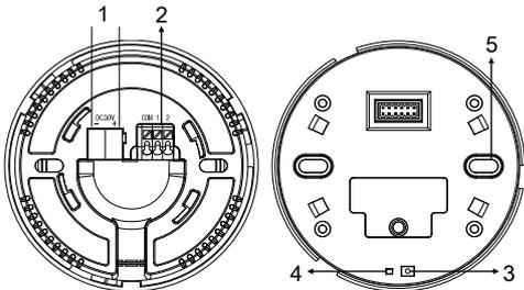
Figure 3. Components - Back View(1) Figure 4. Components - Back View(2)
