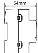
Figure 7. Dimensions - Side View
