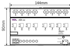
Figure 5. Dimensions - Front View
