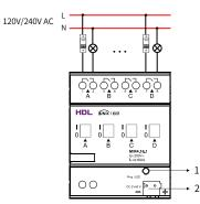
Figure 8. Wiring
