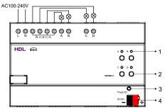
Take the connection of KNX 4CH 1.5A MOSFET Dimming Actuator as an example Figure 8. Wiring
